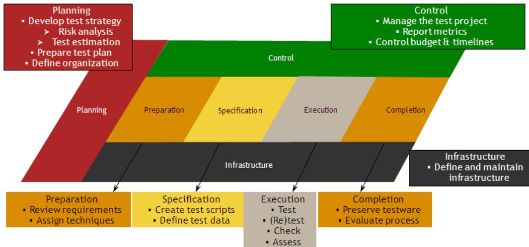
**Figure 6 – TMap Test Life-cycle**
